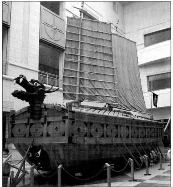
The 1:2.5-scale reproduction turtle ship in the War Memorial Museum, Seoul. This is regarded as the most accurate representation of this famous vessel, showing the two figureheads and the auxiliary sails.
